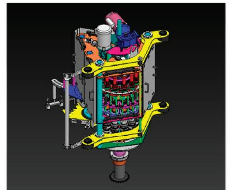
SolidWorks design visualization and motion simulation tools help Fogg Filler efficiently develop large assemblies containing thousands of parts.
